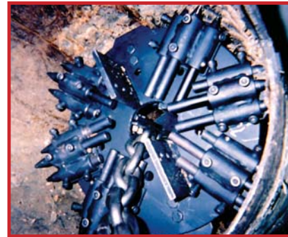
Special tools like this one were used to rip, scrape and scrub collected material from the hospital's medical waste pipe.
