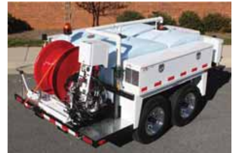
The US Jetting 4018 - 600 unit is an expanded design of the US Jetting 4018-300 with double the water capacity. Identical hose reel & control panel assemblies are used on both units.
