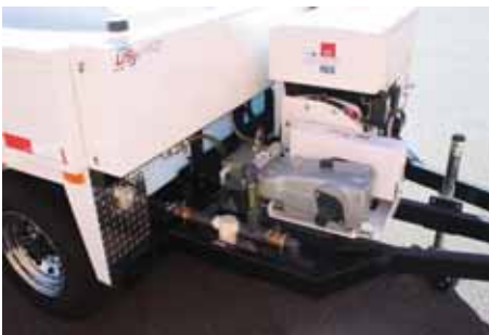
After 20 years, US Jetting 4018 Run Dry Pumps are still powered by a Hatz diesel engines to produce 4,000 PSI at 18 GPM.
