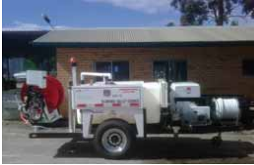
The Clarence Valley US Jetting 4018 -300 Narrow Track Series with optional inlet hose reel.
